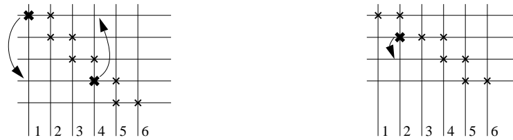
Figure 2: The switch matrix on the left has identical Hamming costs before and after the swap indicated. After the swap, it cannot route any subsets which include wires \{1,5,6\} . Hence, the cost function is not always effective at distinguishing good switch swaps. The switch matrix on the right has lower Hamming cost after the swap indicated, and routes all subsets of size 3. Before the swap it could not route subset \{1,2,3\} . In this case, the cost function can identify a good swap.
