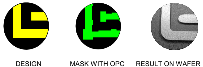
Figure 1: OPC counteracts lithography distortions
