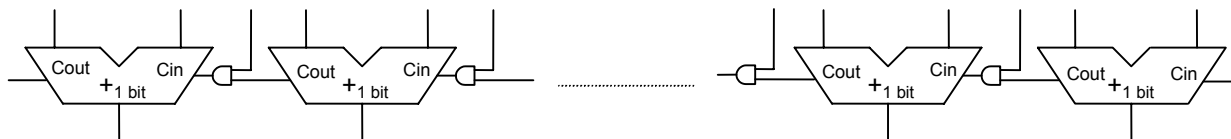
Fig. 3. Array of 1-bit adders linked by 2-input and gates.
