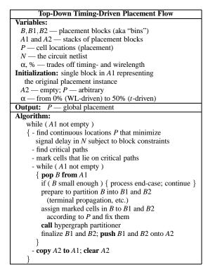
Figure 1: Pseudocode of proposed timingdriven placement framework.
