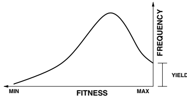
Fig. 3. A noisy development environment leads to a distribution of phenotypic fitnesses. Yield is the frequency with which the distribution reaches the maximum fitness
