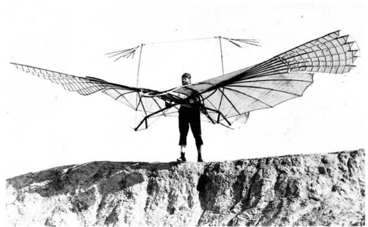
Otto Lilienthal on August 16th, 1894 The glider mimics a bird with spread wing tips
