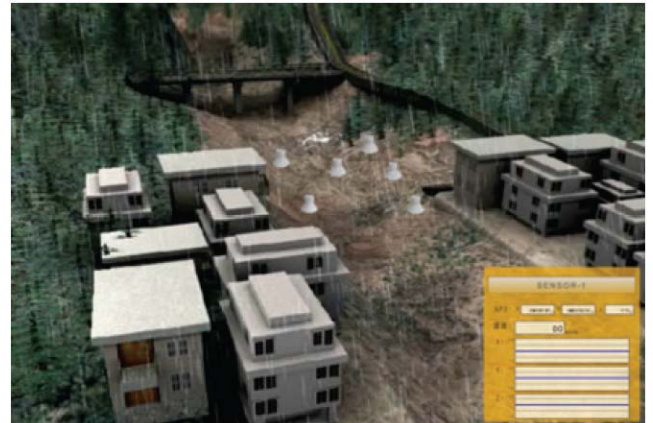
Fig. 1. A group of wireless sensors are scattered deployed on the riverbed for debris flow monitoring.
