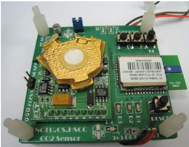
Fig. 7. H-550EV CO 2 sensor integrated with JN5139.
