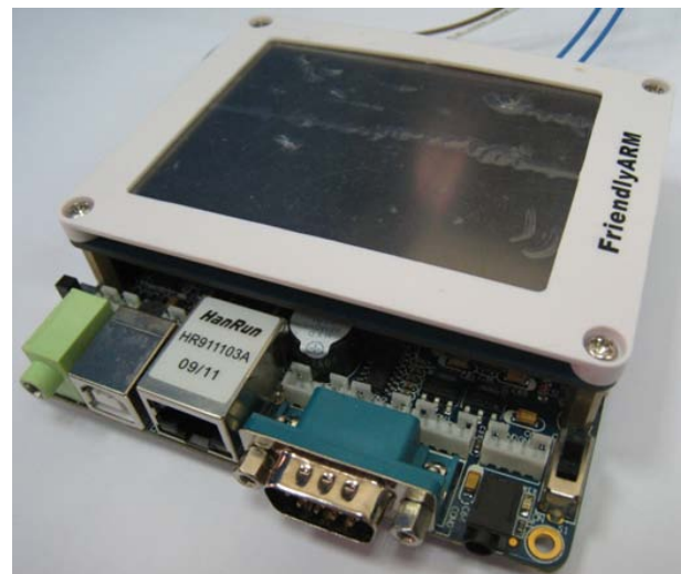
Fig. 6. Mini2440 development board with a 3.5" TFT LCD.
