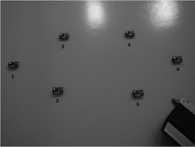
Figure 4: TelosB network setup
